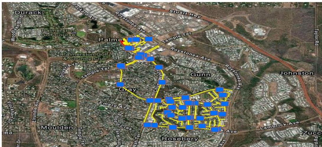
Figure 2 Fibre Sense Pits (Blue) and Fibre Sense Cable (Yellow)
