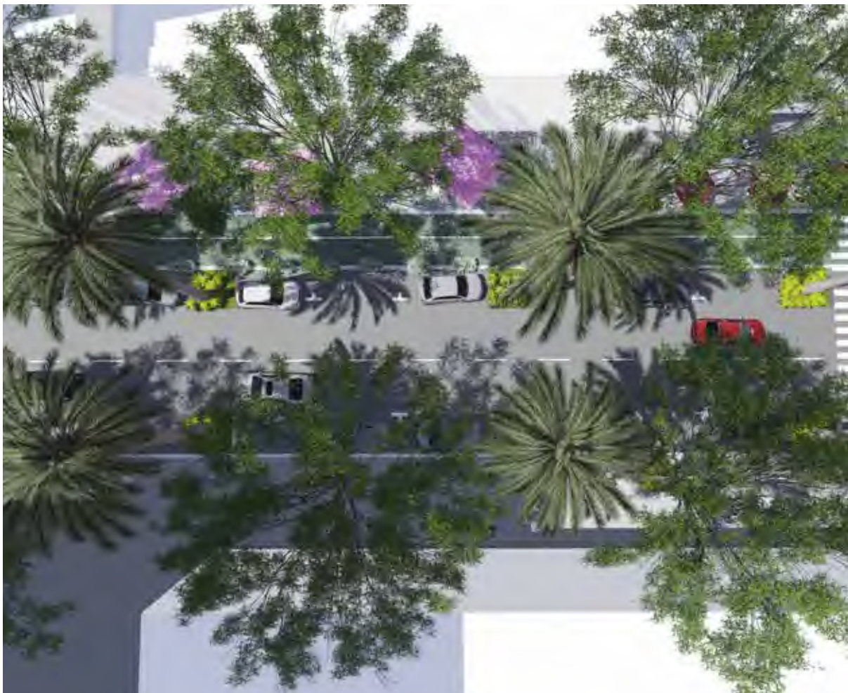
Figure 19. Generous shaded footpaths for solar shading
